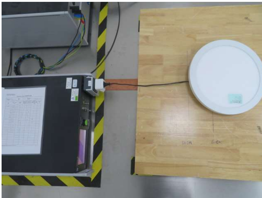
Photograph 4: Set-up for Fast Transient Burst, Surges and Voltage Dips
