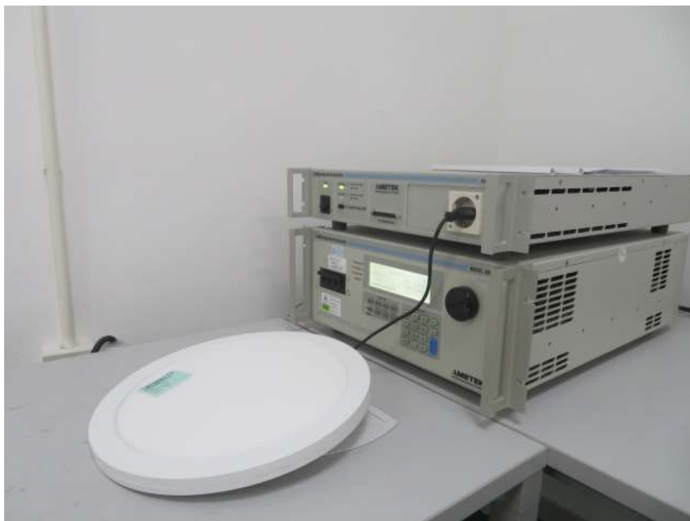
Photograph 8: Set-up for Harmonics
