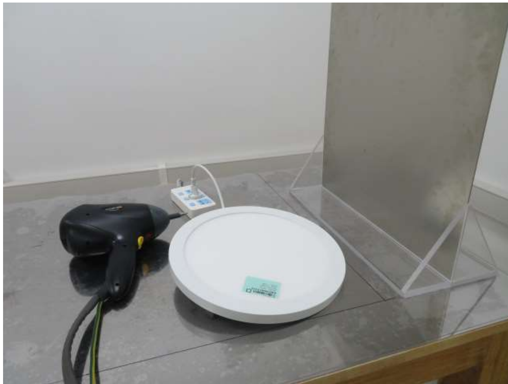
Photograph 4: Set-up for Fast Transient Burst, Surges and Voltage Dips
