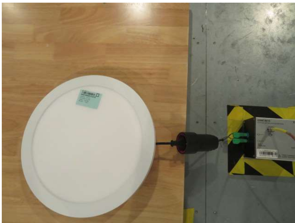
Photograph 2: Set-up for Radiated Emission (CDN Method)
