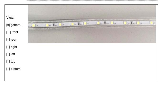
Details of: LED modules view for ST2835-120S-X; model BW2835-120S-X is identical, only different in appearance color.
