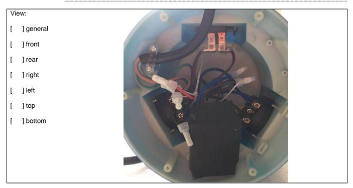
**Detail of:** LED driver for model 30A02A
