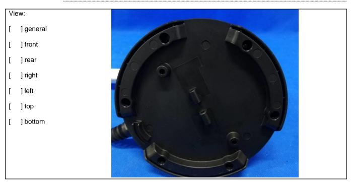
**Detail of:** Cord anchorage for model 31C04
