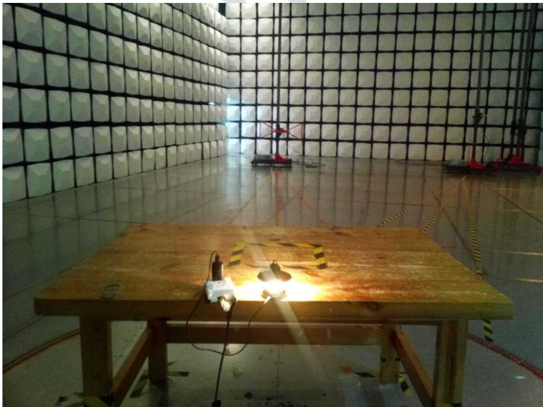
RE Below 1G rear M1 View
