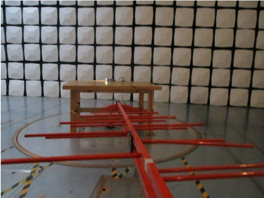
RE Below 1G front View
